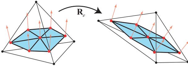
Figure 5: Vertices of the surface mesh (shown in red) are displaced according to the displacement field of the tetrahedron in which they lie. The rotation of the tetrahedron  $\mathbf{R}_e$  is used to rotate the normals.
