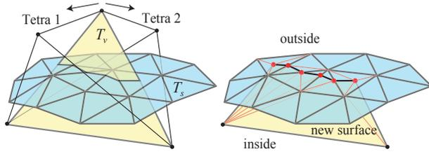
Figure 6: The surface mesh needs to be updated when two tetrahedra that share side  $T_v$  are detached. First, the surface mesh is cut along  $T_v$ . Then, a new surface triangle congruent with  $T_v$  is subdivided along the surface mesh and the triangles that are outside the surface are removed. The ones that are inside are linked to the first tetrahedron and identical copies to the second one.
