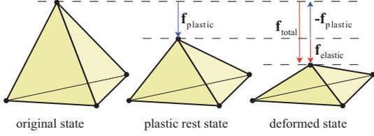
Figure 3: Relative to the original state the deformation of the tetrahedron yields a force of  $\mathbf{f}_{total}$ . In a plastic material only the offset force  $\mathbf{f}_{total} - \mathbf{f}_{plastic}$  relative to the plastic rest state acts as elastic force  $\mathbf{f}_{elastic}$ . Here, the stiffness is chosen such that displacement equals force.
