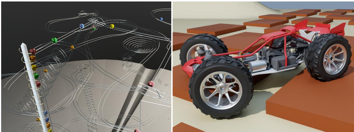
**Figure 1:** Our method allows the stable simulation of a rolling ball sculpture with fast moving marbles and collisions against curved geometry as well as a remote controlled car racing over obstacles with deformable tires.
