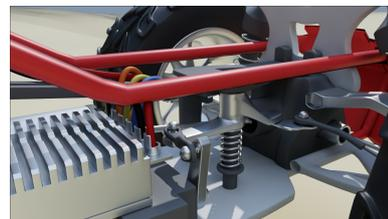
**Figure 16:** We simulate the steering mechanism from the small arm at the servo to the big wheels with a mass ratio of 1:760.
