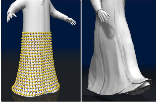
Figure 8: Left: our method creates a single layered simulation mesh for a two-sided visual mesh. Right: simulation of the thick cloth. Model courtesy of CCP.
