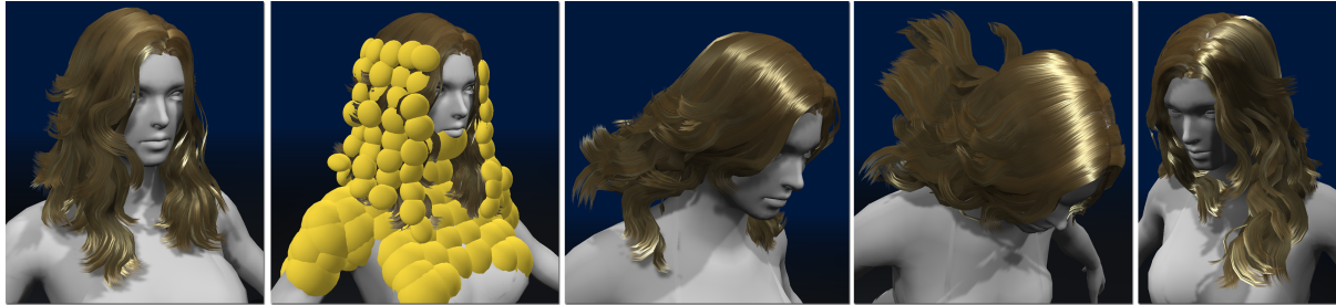
Figure 11: Simulating complex hair geometry with 220 simulation particles for dynamics and collision handling. Model courtesy of CCP.
