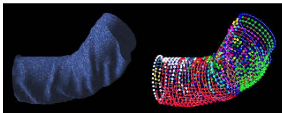
Figure 8: Decomposing cloth into parts which can be solved more efficiently [BA04].
