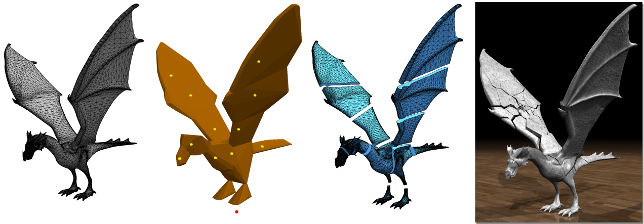
Figure 10: Volumetric Approximate Convex Decomposition of a dragon model with 40k vertices and 80k triangles. Placing twelve nodes intuitively in a matter of seconds results in an tight fitting decomposition that makes fracturing this high resolution mesh possible in real time. From left to right: Original model, compound mesh, one split mesh per convex (shrunk for visualization) and destruction of the model at runtime.
