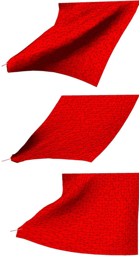
**Figure 3:** Varying the cloth stiffness parameters of different strain components. From top to bottom the resistance to  $x$ -stretch,  $y$ -stretch and shear are: (high,high,high), (high,high,low) and (low,high,high). Our method allows the control of these modes independently on triangle meshes with highly non-regular tessellations as the one used here.
